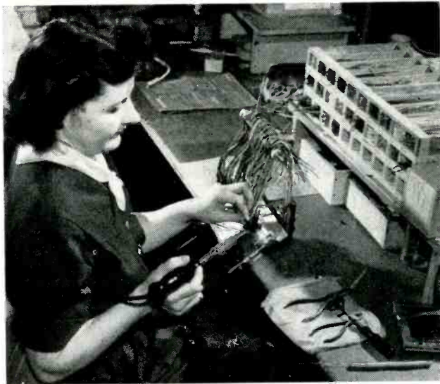
FIG. 7—All plugs are prewired at locations such as these. Note convenient position of operations sheet for quick reference
