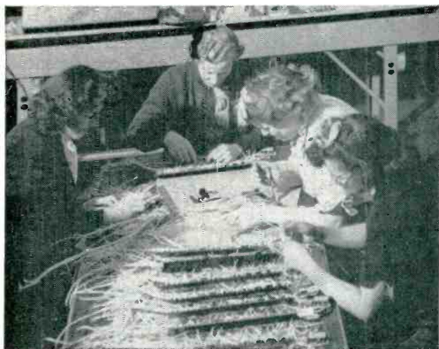
FIG. 5—During World War II, harness making became an important adjunct to equipment fabrication. This photograph shows a typical installation from that period
