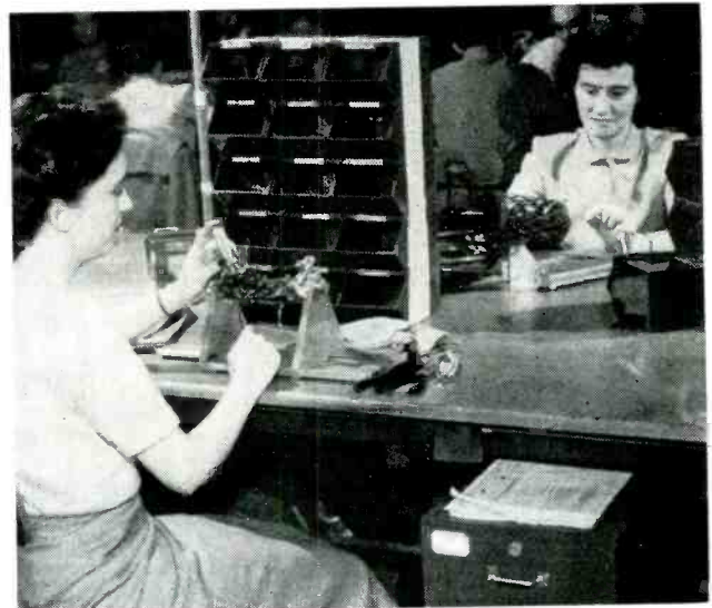
FIG. 8—Subassembly location shows block of stack bins, soldering-iron holder, rubber flap over a-c outlet and tool drawers
