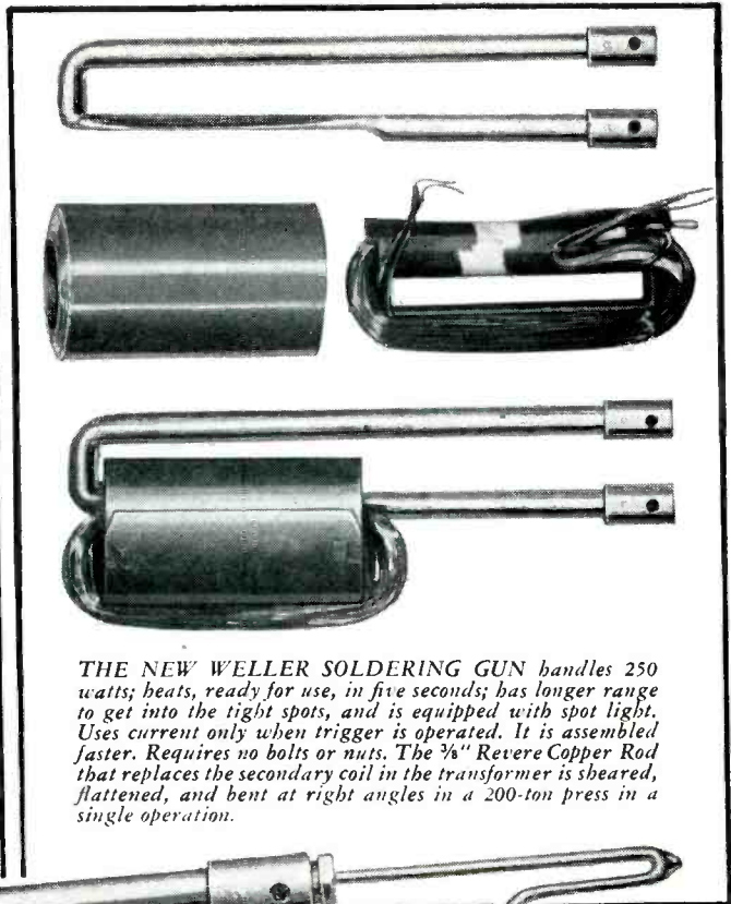
HEAVY, LESS EFFICIENT and slower to assemble, was the original Weller Soldering Gun composed of the parts shown. Compare these with the fewer parts at right in the new Gun, and you'll readily see why the new streamlined Weller is so popular.
