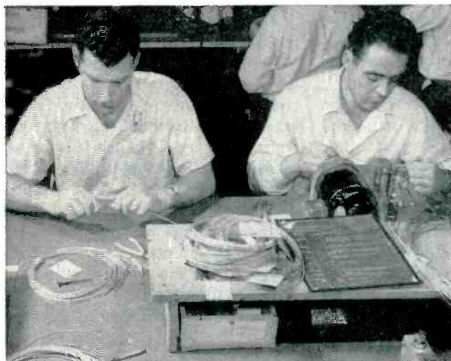
FIG. 3—Production shield-removing operation. At left, operator forms pyramid from shield. Co-worker removes pyramid with nibbling machine so that shield end falls free
